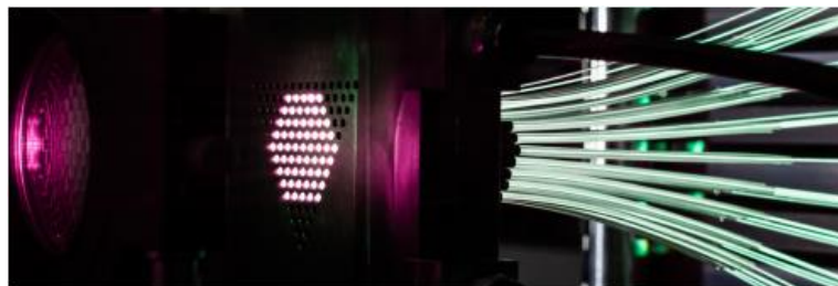
XCAN laser head (center), collimating microlens array (left) and 61 Yb-doped fiber bundle (right) [19].
