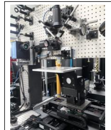
Figure 2: Image of GA-Built Gen-2 (Laser Scanning) 2PP System
