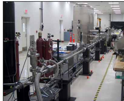
Figure 1: Left: Gas gun for direct drive targets. Right top: Two piece spring loaded sabot that holds target in gun barrel. Right bottom: Sabot in flight being deflected by wedge, allowing the target to continue on the flight path.
