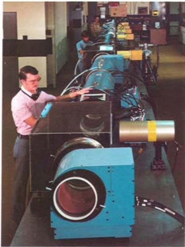
Fig. 16. Cyclops laser chain as viewed from the C-amplifier output stage.
