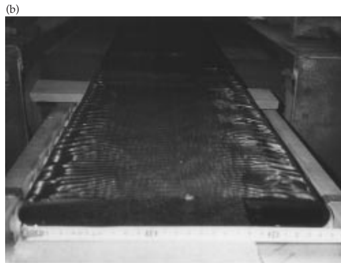
FIGURE 13. Phosphate laser glass formed by Hoya's subscale continuous melter in 1996 at one-fifth NIF scale (a) and at half NIF scale (b). (70-30-0496-0989pb01 top and bottom)
