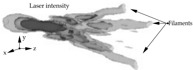
FIGURE 5. Example of a calculation from F3D. The figure shows a constant laser intensity profile for the case where the beam divides into several filaments. (08-00-0896-1888pb01)
