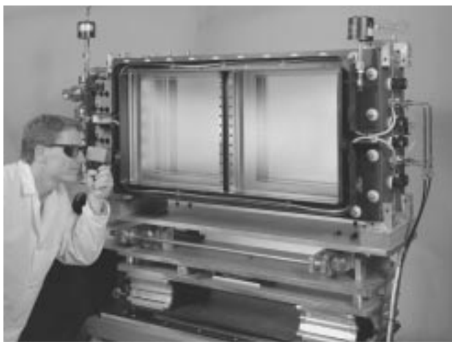
FIGURE 10. A 2 \times 1 prototype of the plasma electrode Pockels cell will test the NIF design. (70-00-0297-0280pb01)
