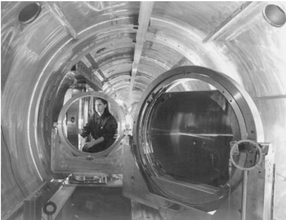
FIGURE 15. Inside the Petawatt vacuum compressor chamber. The two pulse-compression gratings produce a subpicosecond output pulse from a spectrally chirped input pulse more than a thousand times longer in duration. (70-60-0796-1538pb01)
