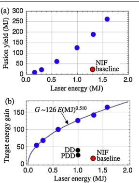
Figure 2. Plot of the one-dimensional (a) fusion yield in MJ and (b) target gain energy versus input laser energy for a family of SI designs, including a NIF (indirect-drive) baseline, a direct-drive (DD), and polar direct-drive (PDD) designs for the NIF, for comparison (from Ref. 11).
