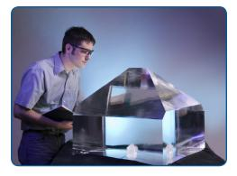
more favorable if the beams are ultraviolet. Passing the laser beams through plates cut from large KDP crystals converts the frequency of their light to ultraviolet before they strike the target. The rapid-growth process for KDP, developed to keep up with
