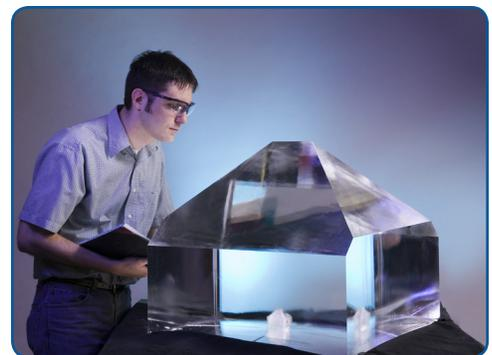
more favorable if the beams are ultraviolet. Passing the laser beams through plates cut from large KDP crystals converts the frequency of their light to ultraviolet before they strike the target. The rapid-growth process for KDP, developed to keep up with
