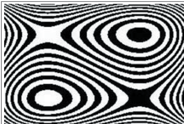
A 100x75 mm phase mask for a discretized \text{mod}(2\pi) diffractive Alvarez lens. This is one of four masks used to create a 16-level kinoform lens.
