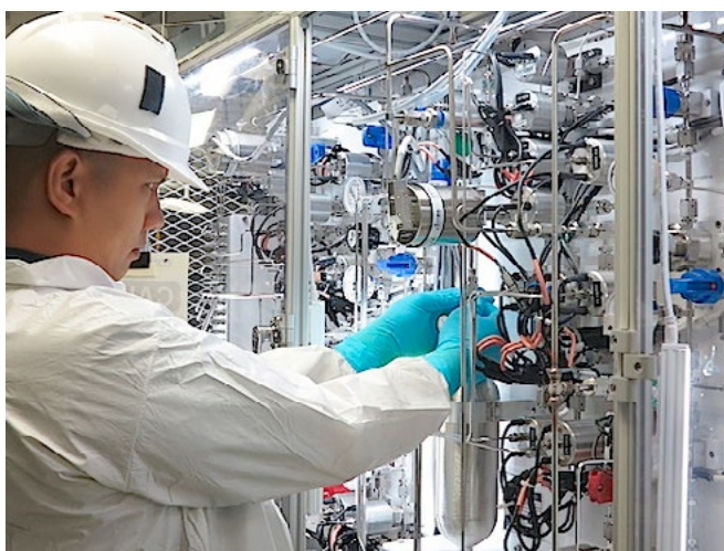
Figure 5-7. Cryogenic System Operator installing a shot gas bottle on a target gas manifold.
