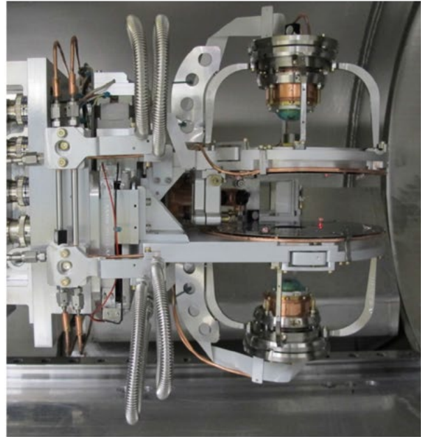
Figure 5-8. Diagram of the Target Alignment Center, showing the three directions for viewing the target (red arrows) and the mirrors for equivalent plane beam alignment.
